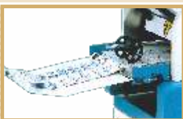
Plain stacker - Horizontal delivery for folded sheets
