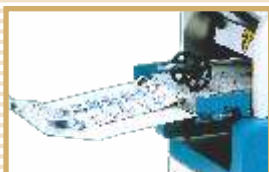
Plain stacker - Horizontal delivery for folded sheets
