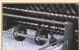
A creasing and perforation attachment at the delivery end
